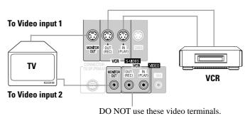
**CASE 4**: If only the VCR is not equipped with the S-video terminal.
